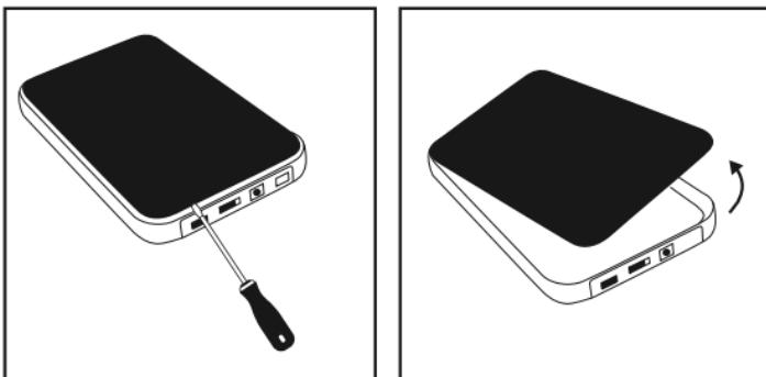
Open the enclosure: hold the silver frame and carefully lever the plate with a screwdriver.
